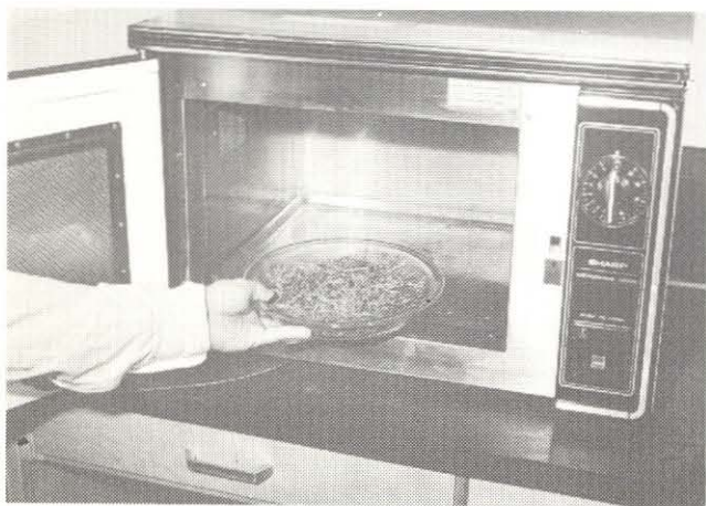
Figure 1. A microwave oven used to estimate moisture levels of alfalfa hay samples
